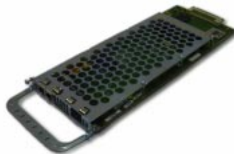
Figure 4 Cisco AS5350 Two-, Four-, or Eight-Port Termination Feature Card
